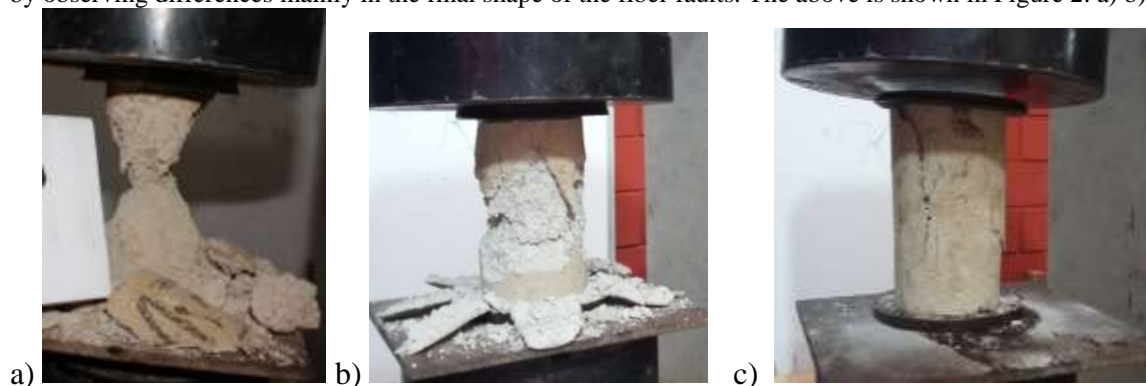
Figure 2.- Samples at the end of test a) of mixtures of Champayan only with water (blank), b) samples with lime and cement and c) mixtures of Champayan with lime, mucilage and fiber.
